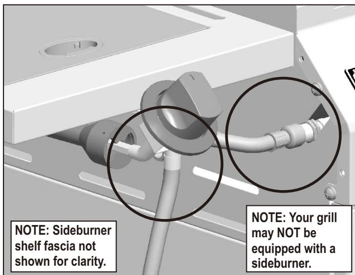
5. If “growing” bubbles appear, there is a leak. Close LP cylinder valve immediately and retighten connections. **If leaks cannot be stopped do not try to repair.** Call for replacement parts.
