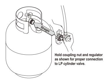
6.Turn the coupling nut clockwise and tighten to a full stop. The regulator will seal on the back-check feature in the LP cylinder valve, resulting in some resistance. An additional one-half to three-quarters turn is required to complete the connection. Tighten by hand only – do not use tools.
