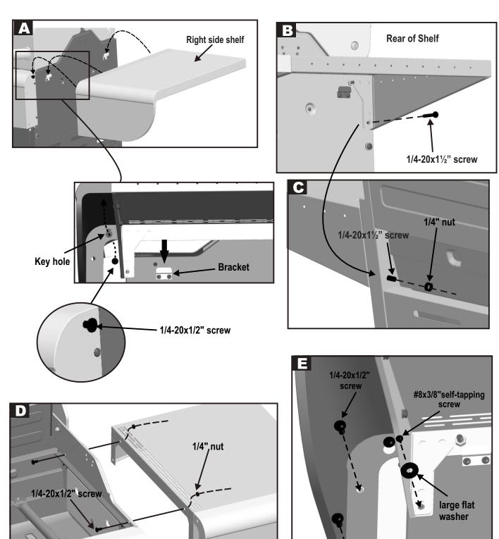
Attach one 1/4-20x1/2" screw to control panel with half of the threads left. Place the key hole slot on fascia onto the screw. Insert flange on left side shelf into side shelf brackets on side of firebox, shown **A**.
