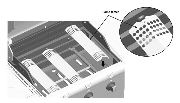
Place infrared emitters onto the firebox as shown. Place one infrared emitter in the middle first.
