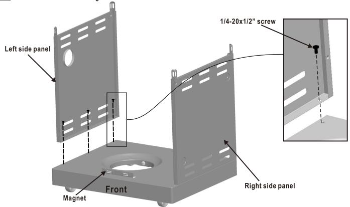
Place lower back panel between side panels at rear of bottom shelf. Secure lower back panel to side panels using two 1/4-20x1/2" screws on each side.
